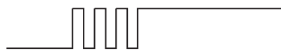
Without a debounce filter, the signal is interpreted to change state multiple times.
